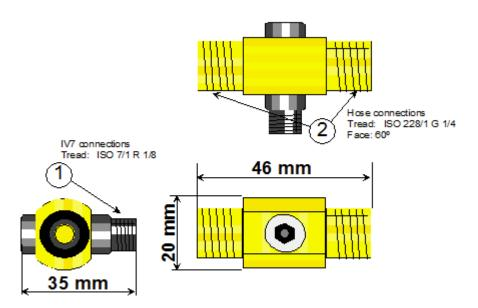
The inlet adaptor is used for connecting hoses for Pneumatic Activation (PA) on Control Inert systems.
