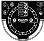
When the field service access door is open, the user has access to the RESET U, DISABLE ■, Fire Test ♠, AutoLearn♦> and Instant Fault Finder functions. When the Instant Fault Finder function is activated, the Smoke Dial™ converts to a fault indicator, with the dial segment numbers corresponding to the faults listed below.
